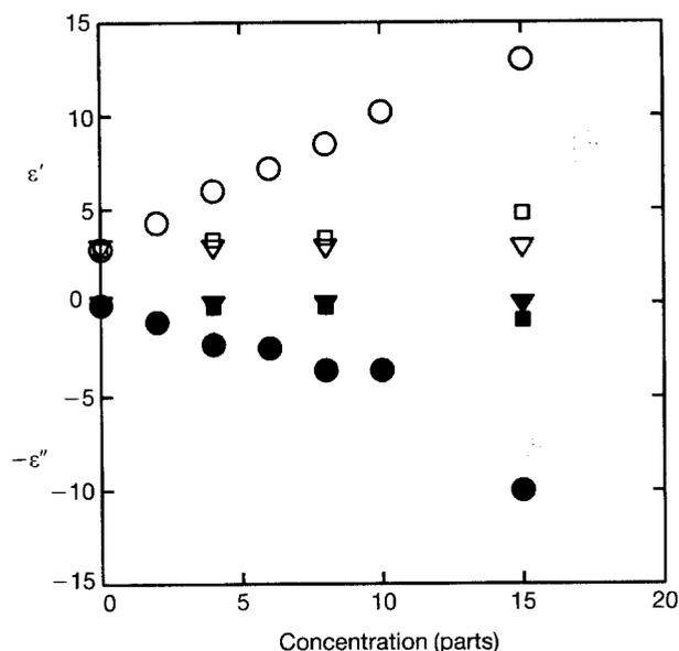
Figure 12 The real part,  $\epsilon'$  (open symbols), and the imaginary part,  $\epsilon''$  (closed symbols), versus concentration of powder in silicone rubber. (○, ●) PPy powder; (□, ■) PAN acid powder; (▽, ▼) PAN base powder.
