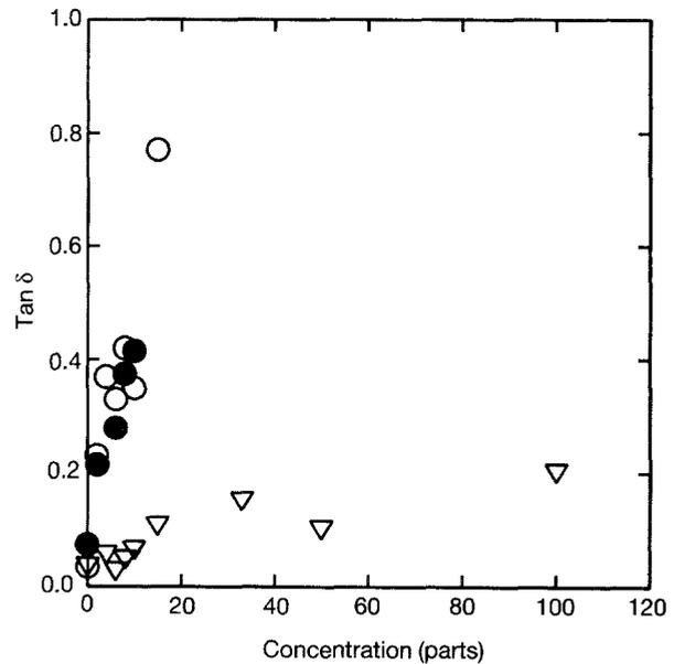
Figure 3 Loss tangent,  $\tan\delta$ , versus concentration of dispersants. ( $\circ$ ) PPy powder/silicone rubber composite; ( $\bullet$ ) PPy powder/vinyl ester composite; ( $\nabla$ ) fully doped PPy/p-TS flakes/silicone rubber composite.
