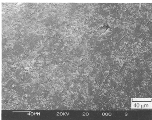
Figure 7 Scanning electron micrograph of PPy powder (15 parts)/vinyl ester composite.
