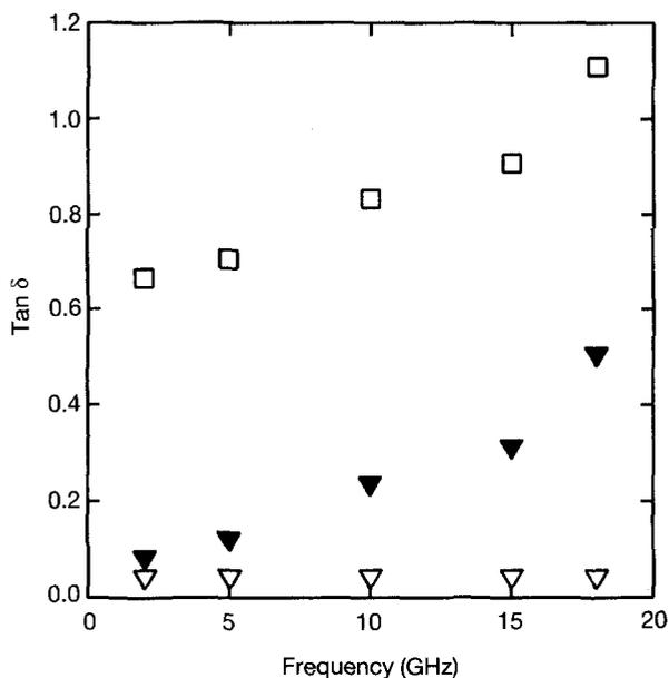
Figure 4 Loss tangent,  $\tan \delta$ , versus frequency. (□) PPy powder (15 parts)/silicone rubber composite; (▼) fully doped PPy/p-TS flakes (100 parts)/silicone rubber composites; (▽) silicone rubber.
