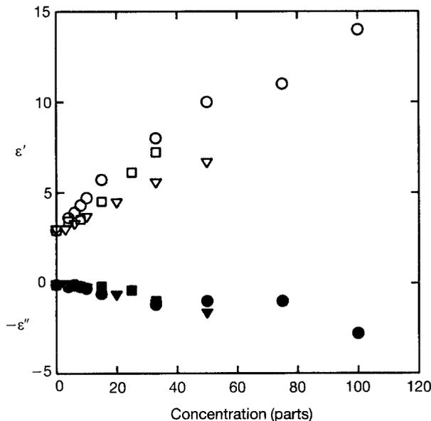
Figure 11 The real part,  $\epsilon'$  (open symbols), and the imaginary part,  $\epsilon''$  (closed symbols), versus concentration of the PPy flakes in silicone rubber. (○, ●) Fully doped PPy/p-TS; (□, ■) PPy/DDS; (▽, ▼) dedoped PPy/p-TS.
