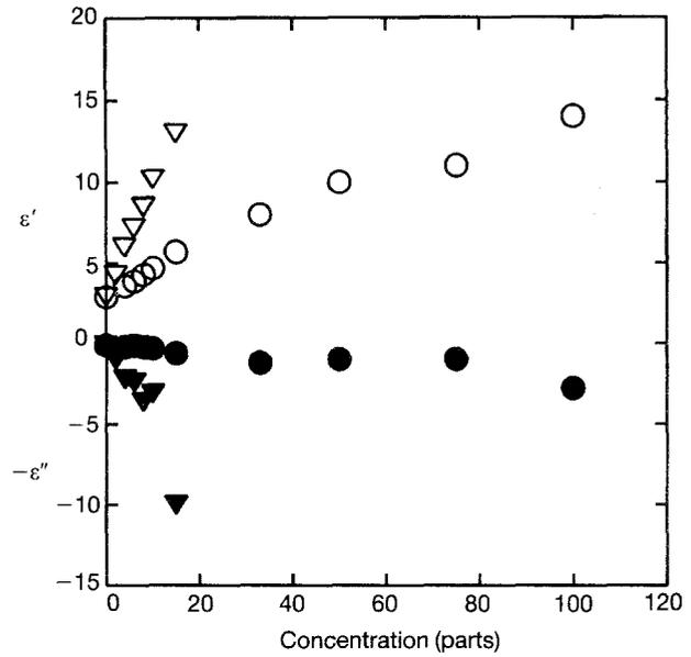
Figure 2 Comparison of the real part,  $\epsilon'$  (open symbols), and imaginary part,  $\epsilon''$  (closed symbols), of the complex permittivity between the PPy powder/silicone rubber and PPy flakes/silicone rubber composites at 10 GHz. ( $\nabla$ ,  $\blacktriangledown$ ) PPy powder/silicone rubber composite, ( $\circ$ ,  $\bullet$ ) fully doped PPy/p-TS flakes/silicone rubber composite.
