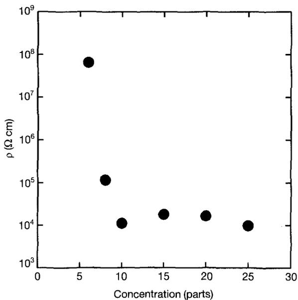
Figure 5 Resistivity,  $\rho$ , versus concentration of PPy powder for the PPy powder/silicone composites.
