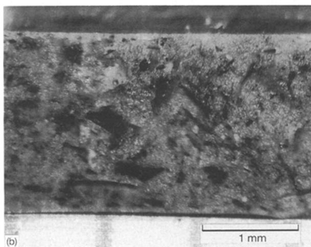
Figure 8 Optical micrographs of fully doped PPy/*p*-TS flakes/silicone rubber composite. (a) 4 parts of PPy flakes; (b) 15 parts of PPy flakes.
