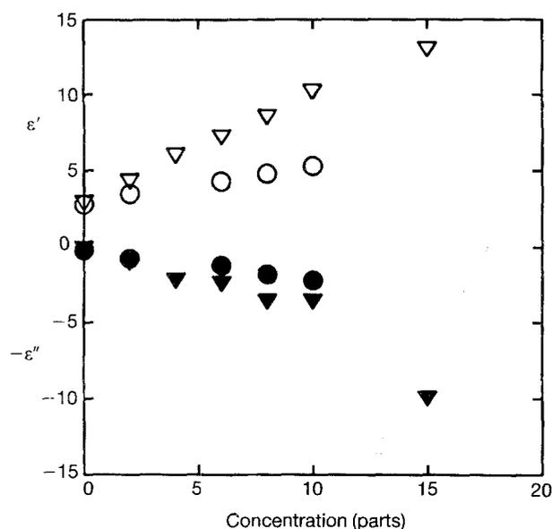
Figure 13 The real part,  $\epsilon'$  (open symbols), and the imaginary part,  $\epsilon''$  (closed symbols), versus concentration of PPy powder in the composites. ( $\nabla$ ,  $\blacktriangledown$ ) Silicone rubber as matrix material; ( $\circ$ ,  $\bullet$ ) vinyl ester as matrix material.
