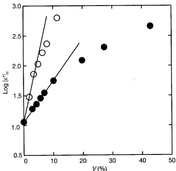
Figure 10 Magnitude of permittivity versus volume fraction. (○) PPy powder/silicone rubber composite; (●) fully doped PPy/p-TS flakes/silicone rubber composite.
