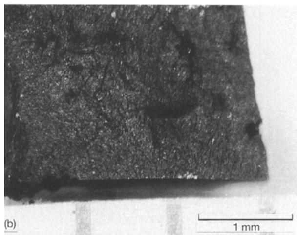
Figure 6 Optical micrographs showing a network of conducting dispersant (dark phase) in PPy powder/silicone rubber composite. (a) 4 parts PPy powder; (b) 15 parts PPy powder.
